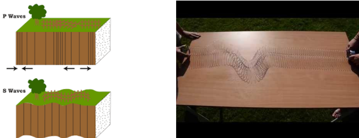
Figure 2: P - waves and S - waves in the crust
