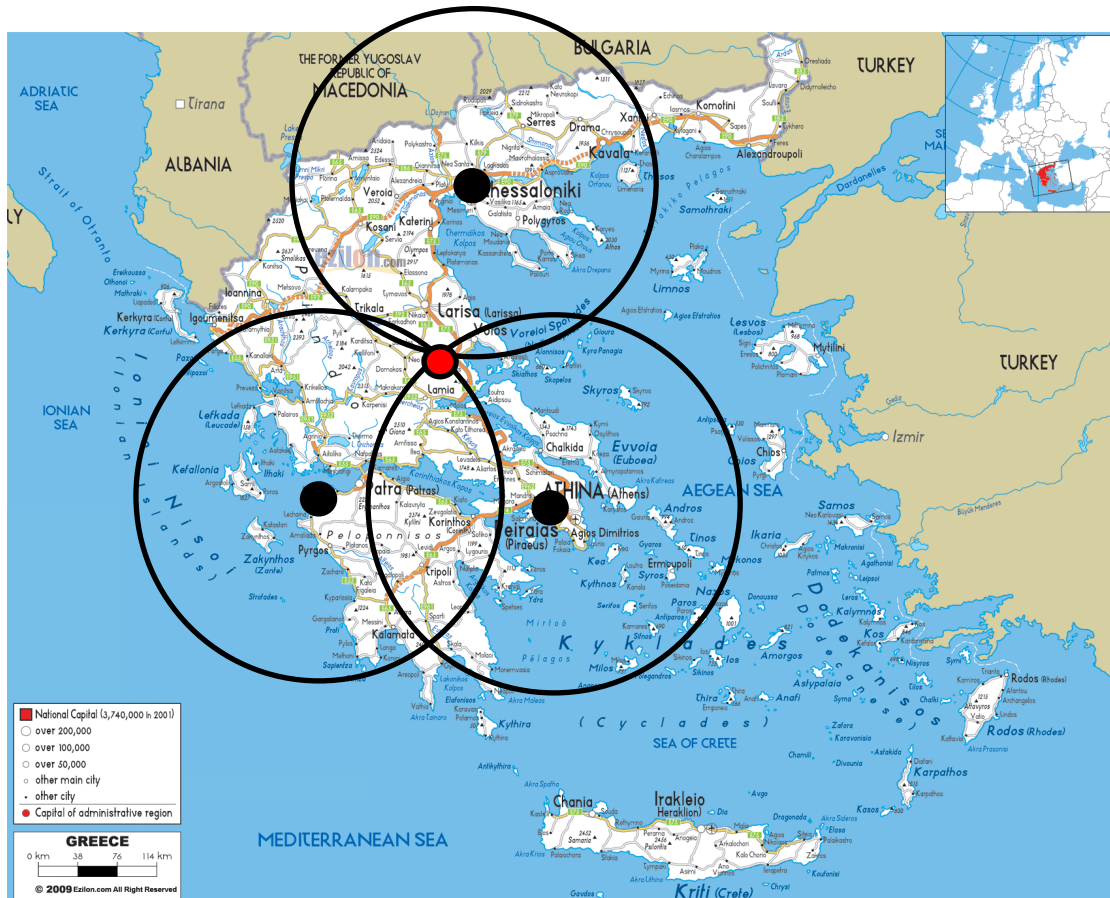
Figure 7. Finding the epicenter of the earthquake using the “triangulation” method. The point where the three circles intersect is the approximate epicenter of the earthquake.
