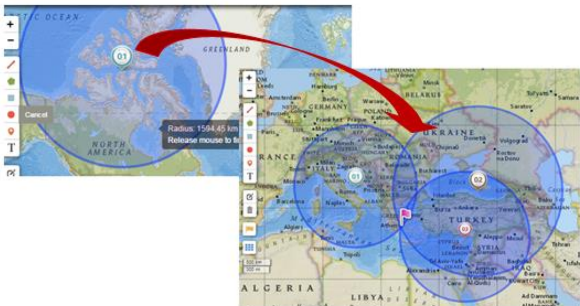
Graph.4: The trilateration technique
